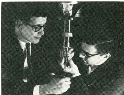
IBM scientists Dr. Peter P. Sorokin (L) and Dr. Mirek J. Stevenson prepare an experiment with a new trivalent uranium optical maser. The trivalent uranium maser emits coherent light waves which have a sharply defined frequency and propagate an intense, directional beam.
