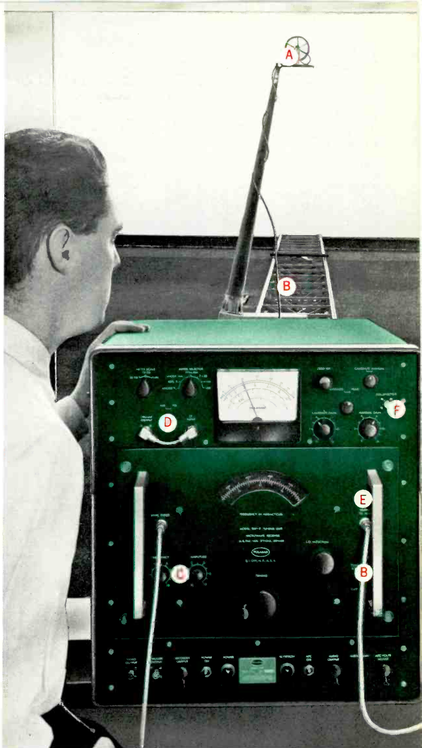
Model RW-T Microwave receiver being used to make antenna pattern measurements on Polarad range.
